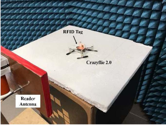
Figure 8. Measurement set up comprising an interrogating linear patch antenna (max gain  $5dBi$ ) connected to the Thing-Magic M6e reader. The sensor-tag onboard the nano-drone was positioned at  $30cm$  distance from the antenna.
