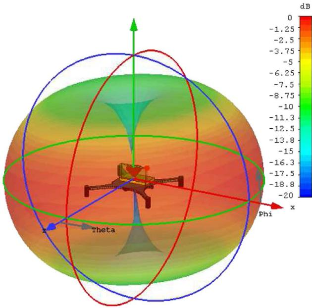
Figure 5. Simulated Radiation gain pattern of the antenna placed under the quadcopter at  $870MHz$ .
