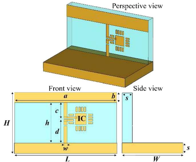
Figure 3. T-shaped tag layout with finite ground plane. Size:  $a = 30 \text{mm}$ ;  $b = 3 \text{mm}$ ;  $c = 4.7 \text{mm}$ ;  $d = 7 \text{mm}$ ;  $w = 1 \text{mm}$ ;  $H = 18 \text{mm}$ ;  $L = 30 \text{mm}$ ;  $W = 15 \text{mm}$ ;  $s = 3 \text{mm}$ .
