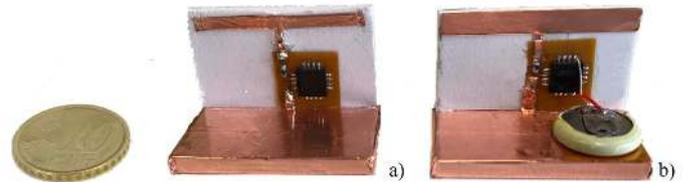
Figure 7. Prototypes of the nano-drone sensor-tag with and without a 3V battery for passive and battery-assisted operations.
