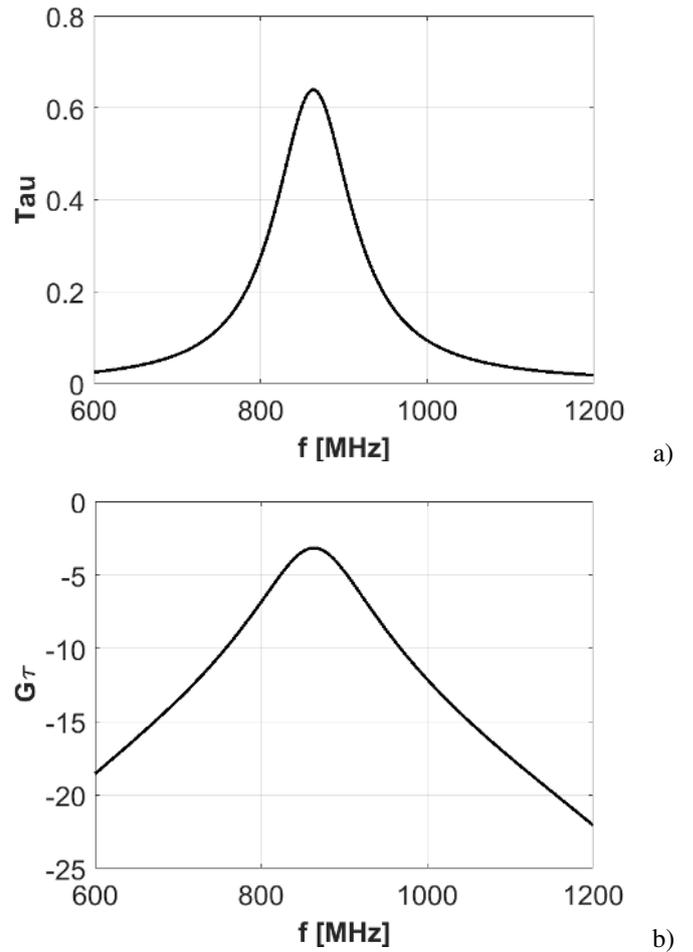
Figure 6. The simulated a) power transfer coefficient and b) the realized gain of the tag antenna when mounted onboard the nano quadcopter.
