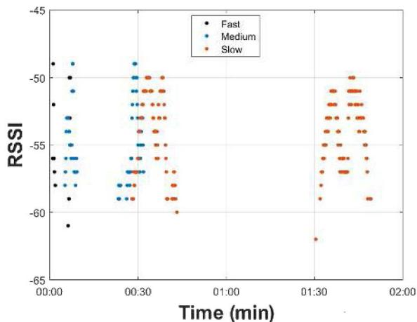
Figure 11. The RSSI values returned by the battery-less Tag-Drone flying along the guiding rails from the floor (position A), up to the ceiling (position C), passing in front of the reader's antenna (position B) where the RSSI peak occurs, and downhill. a) Fixed velocity  $v = 0.05m/s$  and different reader-rails distances; b) fixed reader-rails distance  $d = 1m$  and different speeds.
