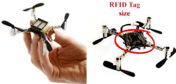
Figure 2. The Crazyflie 2.0 reference quadcopter with indication of the place where the tag antenna will be placed.
