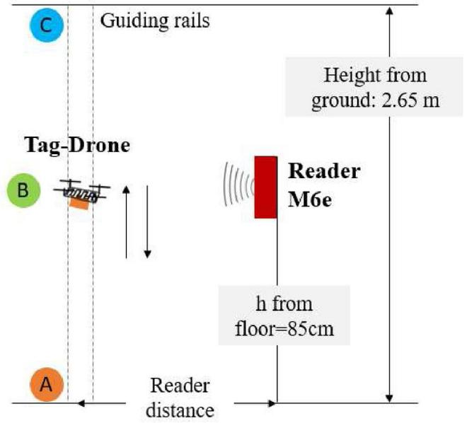
Figure 10. Schematic of the experimental setup for the evaluation of the RFID link by a flying tag constrained to move along vertical wired rails.
