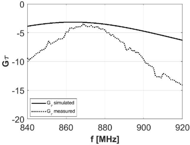
Figure 9. Measured and simulated realized gain of the Tag-Drone in frontal direction.
