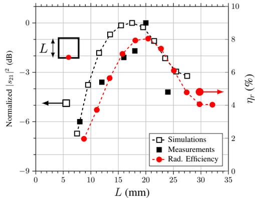
Fig. 2. Comparison between measured and simulated normalized gains of the 3.6 GHz epidermal loop and radiation efficiencies  $\eta_r$  as function of  $L$ . Inset: in-scale view of the 3.6 GHz loop, size:  $17.5 \times 17.5 \text{ mm}^2$ .
