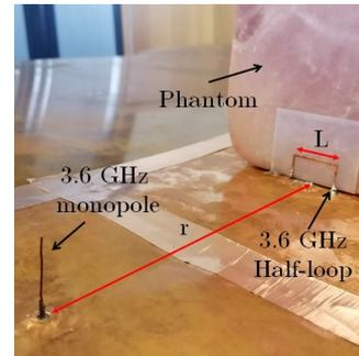
Fig. 1. Experimental setup for measuring the gain of the 3.6 GHz epidermal half-loop when attached onto a roasted pork phantom.
