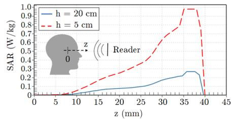
Fig. 3. SAR distributions from a source emitting 4 W EIRP at 5 and 20 cm away from the face. Results are below the FCC requirements of  $1.6 \frac{\text{W}}{\text{kg}}$  averaged over 1 g of tissue.
