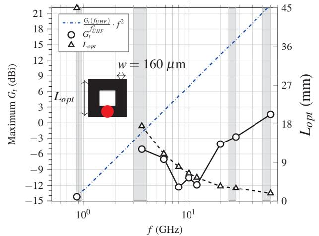
**Figure 1.** Simulated optimal gains of epidermal loops on skin. The 5G frequency bands are shaded in gray. The dashdotted line displays the theoretical  $G_t(f)$  required to keep unchanged, at every frequency  $f$ , the tag read distance.
