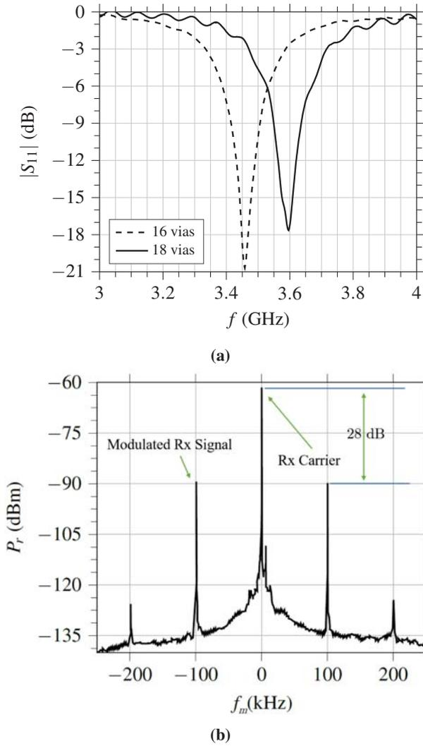
**Figure 4.** (a) Power reflection coefficients of the reference patch antenna. Tuning through vias is highlighted. (b) Received spectrum upon backscattering.  $r = 15$  cm,  $P_m = -30$  dBm. Modulation:  $f_m = 100$  kHz,  $V_{pp} = 750$  mV, DC offset = 375 mV.
