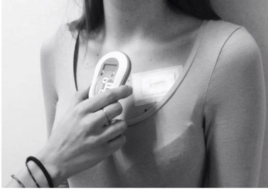
Figure 4. Epidermal plaster on the human chest wirelessly read by an handheld reader.
