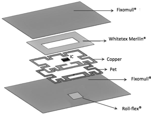
Figure 1. Sketch of the various layers of the reusable epidermal RFID thermometer.
