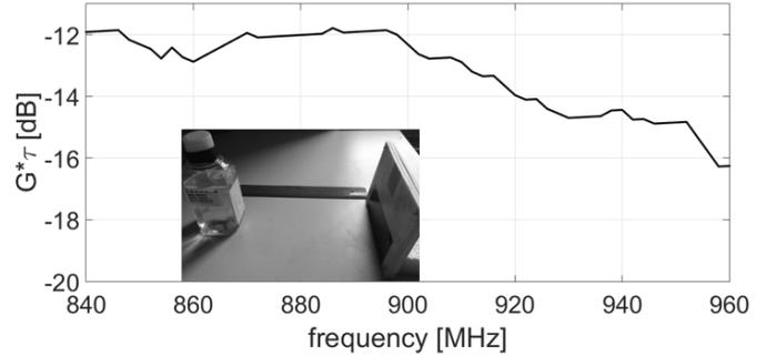
Figure 3. Measured realized gain of the passive epidermal thermometer placed over a liquid phantom..
