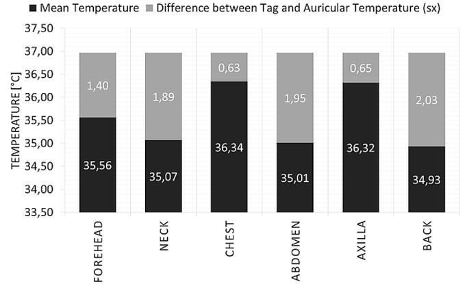
Figure 6. Mean skin temperature recorded by the epidermal thermometer over different body positions (Fig.I) and difference with respect to the tympanic temperature.
