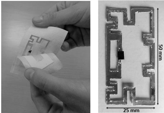
Figure 2. Sterile battery-less epidermal thermometer made of disposable dressings and a reusable inner transponder.
