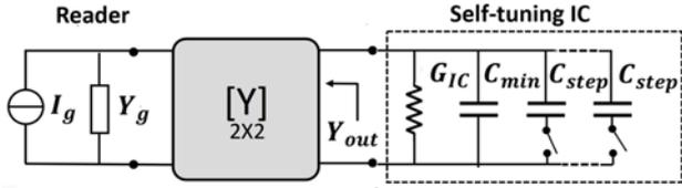
**Figure 2.** Two-port network model of the fingertip-reader link where the self-tuning IC is modeled using a variable capacitance whose value is a dynamic function of the susceptance  $B_{out}$  seen from the IC terminal.
