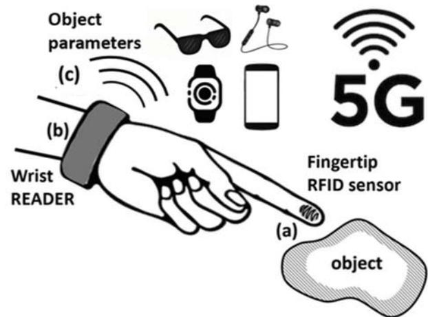
**Figure 1.** Sketch of an R-FAD system comprising a fingertip RFID sensor tag (a) which is coupled in near-field with a wrist-worn reader (b) and returns some measured parameters of the touched object via backscattering modulation. The object parameters (c) are then sent by the wrist reader to a body-worn device (smartphone, earphones, smartwatch or smart glasses) via 5G, ensuring the low latency required by Tactile Internet.
