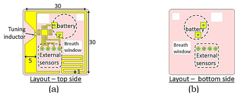
**FIG. 1** – Layout of the RFID skin board: (a) main side with the antenna traces and (b) opposite side with replicated pads. Main sizes in [mm].
