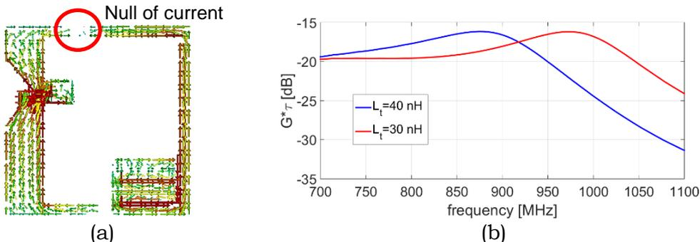
**FIG. 2** – (a) Surface current of the epidermal antenna at 868 MHz and (b) numerically evaluated realized gain for two values of the tuning inductors.
