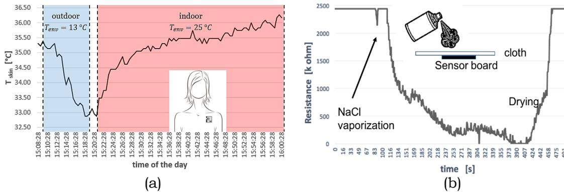
**FIG. 4** – (a) Temperature profile moving from outdoor to indoor environment. (b) Surface resistance of a cloth that was humidified by physiologic solution.
