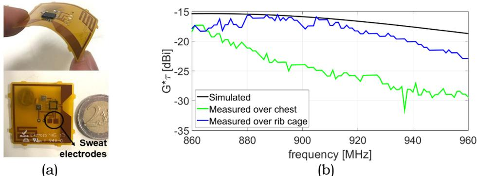
**FIG. 3** – (a) Front and rear sides of the RFID Epidermal Sensor Board prototype with battery mounted onto different faces and (b) measured realized gain when it was placed onto both chest and rib cage of a volunteer.
