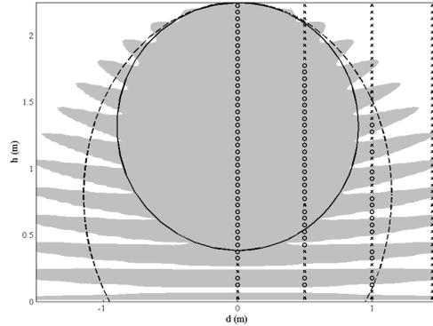
Fig. 3 Interrogation region prediction in case of the reader's antenna pointing toward the ground. Comparison between free-space model (dotted line ellipse), two-rays model (continuous line ellipse), full ray-tracing (gray region) and measurements shown by means of circle and cross markers. Circles concern reading locations, crosses non-reading locations. Reader power: 1.2 W EIRP
