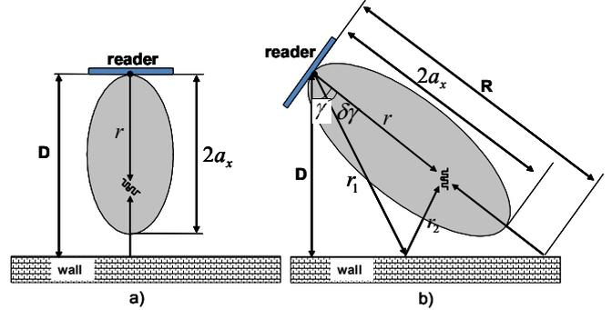
Fig. 2 Ellipsoid model of read-region (dark area) of a reader antenna in front of a wall. a) orthogonal incidence; b) oblique incidence
