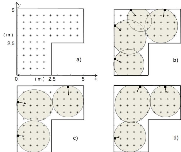
Fig. 4 L-shaped environment wherein network coverage is planned with different constraints. a) set-up with {rT} shown by crosses; b) EIRP and antennas orientation (indicated by arrows) optimized; c) number of readers, EIRP and orientation optimized; d) complete optimization, where also the position of readers is optimized. Arrows show antennas' orientation, ellipses interrogation region. The size of an ellipse is related to the radiated power and to the beam-width of the antenna.
