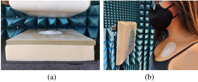
Fig. 10. Measurement setup in a semi-anechoic room. CP reader antenna at fixed distance of 10 cm. (a) Prototype attached on a semi-solid three-layers phantom. (b) Volunteer wearing the device on the chest.
