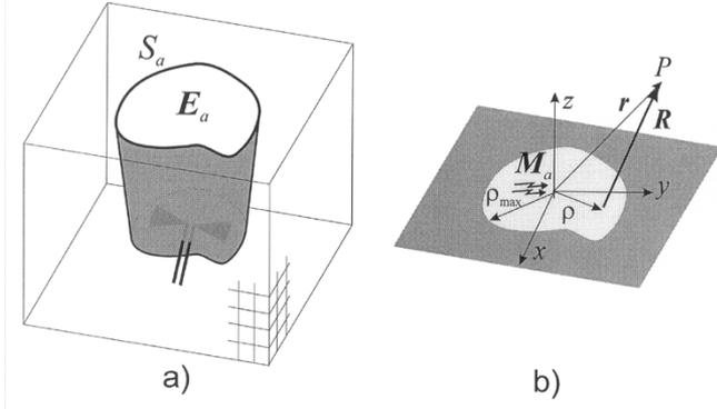
Fig. 1. Strategy for aperture-antenna modeling: (a) the aperture field  $\mathbf{E}_a(\boldsymbol{\rho}, t)$  is computed by a local method applied to a limited space region; (b) the aperture radiation is calculated for the simplified model of an equivalent magnetic source  $\mathbf{M}_a(\boldsymbol{\rho}, t) = \mathbf{E}_a(\boldsymbol{\rho}, t) \times \hat{\mathbf{z}}$  on an infinite screen.
