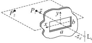
Fig. 2. Dipole-sourced rectangular slot on an infinite ground plane. Size (in centimeters):  $a = 10$ ,  $b = 5$ ,  $L_d = 11.5$ ,  $z_d = 8$ .
