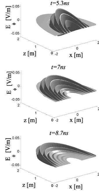
Fig. 4. Radiation from a dipole-sourced rectangular slot on an infinite ground plane, for different times and for  $r > 0.5$  m.
