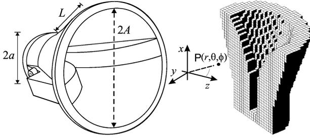
Fig. 6. Circular ridged horn for 4 GHz – 10 GHz frequency band. Sizes (in centimeters):  $A = 3.6$ ,  $a = 1.8$ ,  $L = 6$ ; FDTD model on a cubic grid (half the geometry has been removed for clarity).
