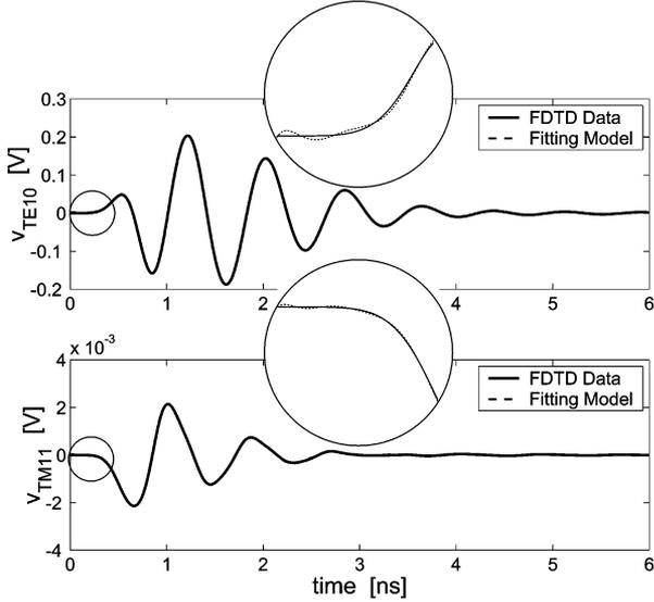
Fig. 3. Fitting of slot modal voltages  $v_{TE_{10}}(t)$  and  $v_{TM_{11}}(t)$  by means of (4) with eight and 11 poles, respectively. The very early transient is magnified within circles.
