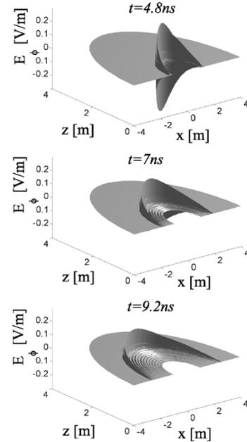
Fig. 9. Snapshots of CRH far field  $E_\phi$  on the H-cut, computed by the new method at different times for  $r > 1$  m.
