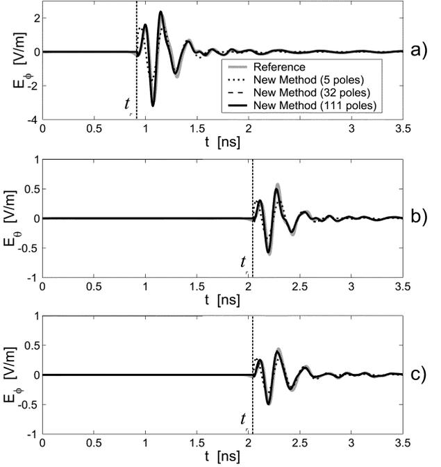
Fig. 8. Transient radiated electric field from CRH antenna computed by full FDTD model (reference) and generated by means of different numbers of poles corresponding to  $\varepsilon = 10^{-1}$ ,  $\varepsilon = 10^{-2}$  and  $\varepsilon = 10^{-3}$ ; (a)  $E_\phi$  at point  $P_1$ , (b)  $E_\theta$  at point  $P_2$ , c)  $E_\phi$  at point  $P_2$ .
