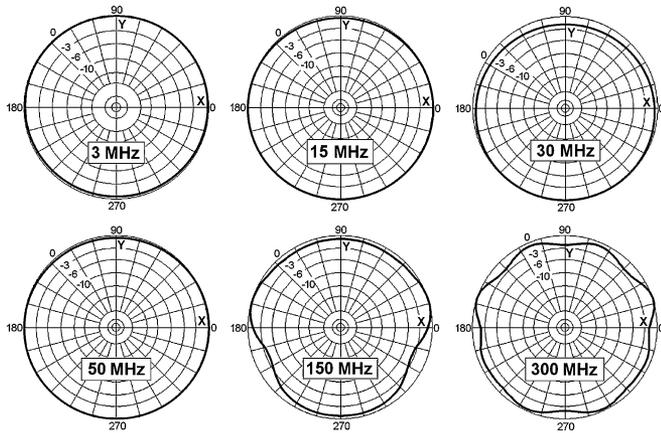
Fig. 7. Normalized horizontal gain with respect to the maximum value at different frequencies for the integrated antenna system in Fig. 3. The structure is placed as in Fig. 1 with respect to the reference axis.
