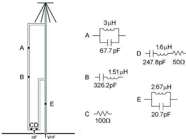
Fig. 3. Reoptimized bifolder-loading configuration. An LC-parallel circuit (tagged by "E") was selected by the GA on the right vertical conductor. When using a coaxial cable of diameter 5 mm, for instance, the inductance in the circuit "E" corresponds to a coil of ten turns, of length 10 cm and diameter 5 cm. The HF transformation step-up ratio was set to 4 as in [4].
