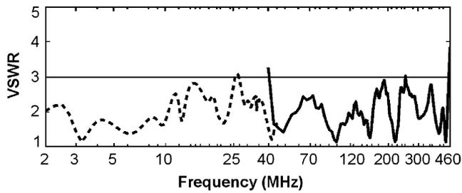
Fig. 6. VSWR of the integrated antenna system in Fig. 3 in the overall 2–440-MHz range. Bifolded VSWR (dotted line) was extended up to 45 MHz.
