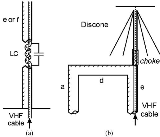
Fig. 2. (a) Inductor of the LC-parallel circuit is obtained by twisting the VHF cable itself. (b) HF-choke used to suppress the induced currents on the discone antenna.
