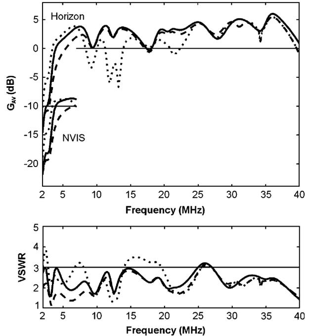
Fig. 4. HF performances:  $\phi$ -averaged gain at horizon ( $\theta = 90^\circ$ ) and NVIS ( $\theta = 20^\circ$ ) and VSWR of the following antenna systems: standalone reoptimized bifolder (solid line), unchoked bifolder + discone (dotted line), bifolder + discone and finite impedance model ( $|Z_s|/s\Omega = 500\Omega$  as in [10]) for the HF-choke in Fig. 2(b) (dashed line).
