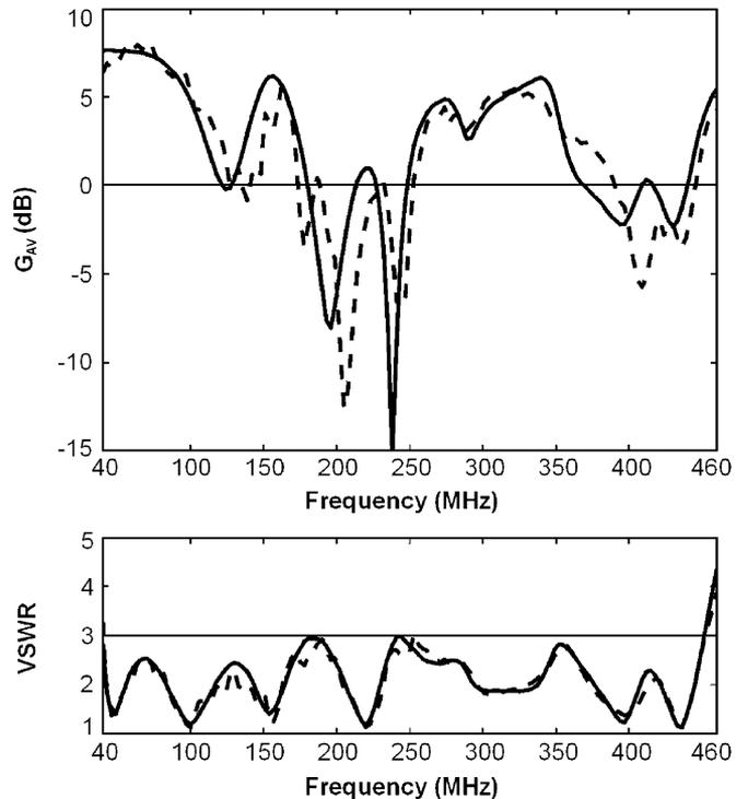
Fig. 5. VHF performances: VSWR and  $\phi$ -averaged gain at horizon ( $\theta = 90^\circ$ ) of the discone antenna in two different configurations: discone on the bifolder in Fig. 3 (dashed line), and standalone discone placed at the same height from the ground plane (solid line).
