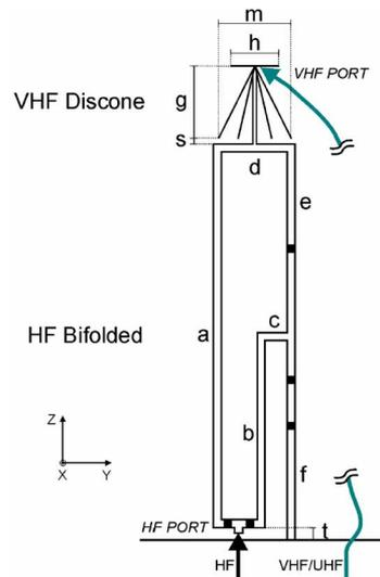
Fig. 1. Two-ports antenna system obtained by combining the bifolded and the discone radiators. Dimensions (in meters):  $a = 12$ ,  $b = 6$ ,  $c = 0.8$ ,  $d = 2$ ,  $e = 6$ ,  $f = 6$ ,  $g = 2.17$ ,  $h = 1.55$ ,  $m = 1.9$ ,  $s = 0.2$ , and  $t = 0.4$ . Bifolded pipes diameter = 0.1. Discone wires diameter = 0.004. Black squares indicate the impedance loads in the original bifolded monopole design in [4].
