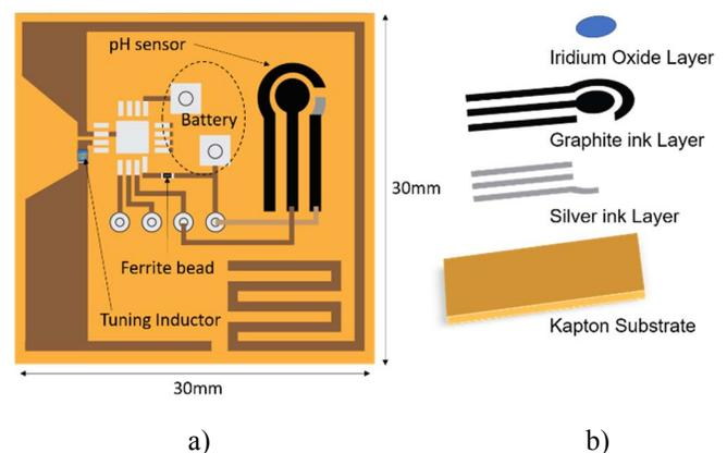
Figure 1. a) Layout of the UHF pH sensor including a thin Kapton substrate, an open coil harvester, a microchip providing ADC and modulation capability and b) a printed multi-layer chemical sensor.
