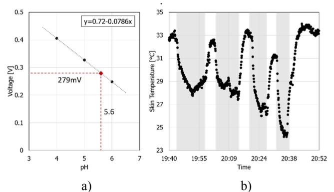
Figure 3. a) calibration curve of the pH sensor; b) temperature data during a 30 min jogging task (grey areas) outside (average temperature  $13 \text{ }^\circ\text{C}$ ), alternating rest periods.
