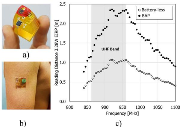
Figure 2. a) Prototype of the UHF pH sensor; b) on-arm placement by Tegaderm™ film; c) read distance measurement for 3.2 W EIRP interrogating power.
