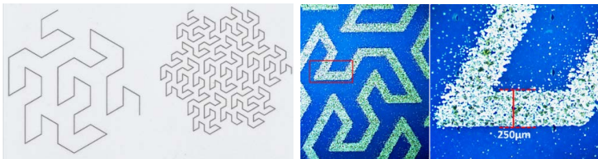
FIG. 3 Some inkjet-printed Gosper SFCs, with a trace 250 \mu\text{m} of increasing orders, over a PET substrate (left). Magnified photo of the n=4 curve (right).
