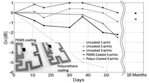
Figure 10. Variation of the maximum realized gain v.s. time of bare tags (single and overprinted) and coated tags with the respect of the initial value (printing time,  $t=0$ ).
