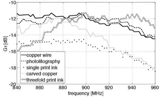
Figure 12. Measured Realized gains (broadside direction) vs. frequency of the epidermal tags attached over a volunteer's arm as in Fig. 11.
