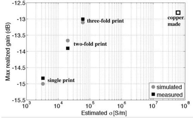
Figure 6. Maximum realized gain (measurements and simulations) of epidermal tag at 900 MHz as function of the estimated ink conductivity.
