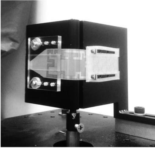
Figure 8. Ink-jet printed antenna mounted over a hinge set-up for the bending fatigue test.
