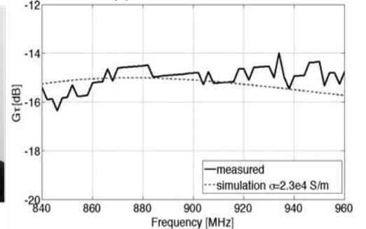
Figure 5. a) Inkjet-printed meandered-loop epidermal antenna over PET substrate. b) Simulated and measured realized gain (broadside direction) when the tag is attached onto a liquid phantom simulating the human body.
