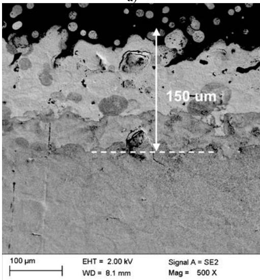
Figure 4. SEM micrographs a) (100Kx) showing the macrostructural evolution of the granular conductive patterns as a function of the number of printing passes. b) 500x magnification of the trace edge in case of four-pass printing
