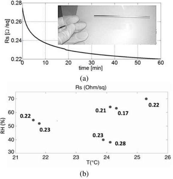
Figure 1. a) Time-variant dc sheet resistance (in  $\Omega/\text{sq}$ ) of a printed  $W/L=100$  trace on PET transparent film as measured at ambient conditions ( $T = 24.1^\circ\text{C}$  and relative humidity  $RH = 64\%$ ). Time  $t=0$  marks the end of the print procedure. b) Sheet resistance of several printed traces on PET for variable ambient conditions during the printing process.
