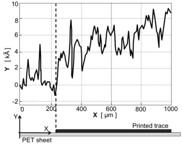
Figure 2. Measured profile (by Dektak 3ST surface profilometer) of the inkjet printed trace on PVA-coated PET film.
