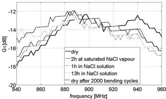
Figure 9. Measured realized gains of a threefold printed epidermal antenna before and after exposure to 100% RH, after immersion in saline solution and after 2000 of bending cycles.
