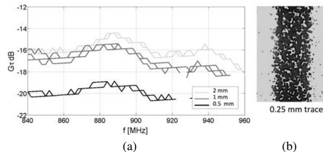
Figure 7. (a) Measured realized gain of three couplets of epidermal antennas made by different trace width  $w = \{2, 1, 0.5, 0.25\}$  mm. (b) Magnified details (60x) of the 0.25 mm highly porous single-printed trace.
