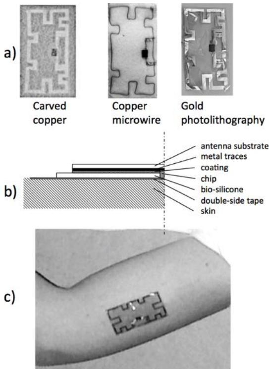
Figure 11. a) Prototypes of the test antenna made for comparison by three different manufacturing technologies; b) (half) cross-section of the corresponding integrated plasters. Depending on the antenna technologies, the *antenna substrate* is PET (inkjet), polyimide (photolithography) or biosilicone (copper-based methods) c) example of the placement over a volunteer's arm.
