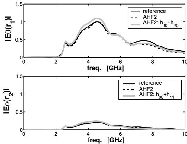
**Figure 11.** CRH antenna: comparison between reference solution and AHF2 reconstructions for the far-field data (normalized units) at the boresight,  $P_1 = (r_1 = 15$  cm,  $\theta = 0^\circ$ ,  $\phi = 0^\circ$ ), and off-the-boresight,  $P_2 = (r_2 = 48.8$  cm,  $\theta = 18^\circ$ ,  $\phi = 45^\circ$ ).
